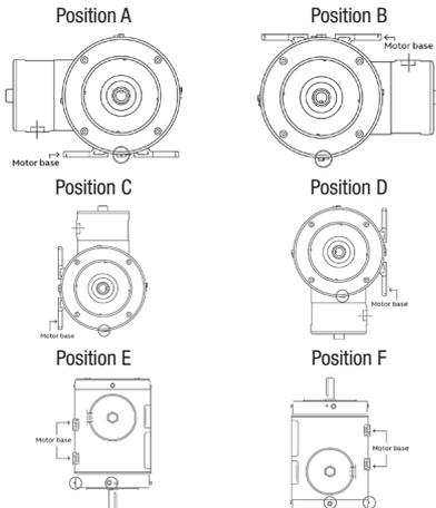
Positions A, B, C, D: leave drain open or install T'drain at both ends of the motor at circled locations. Plug all other drain holes. Positions E, F: leave drain open or install T'drain at circled locations. Plug all other drain holes.
